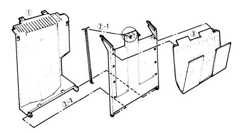
1 Slide the metal tabs on the copy tray into the slots in the bottom of the machine.
